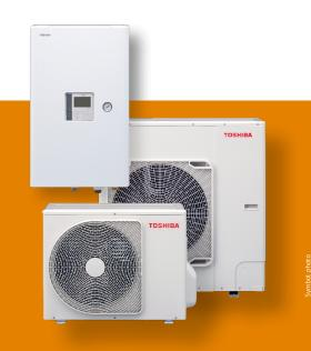
R32 Air to water heat pumps in split design for leaving water temperatures up to +65°C, in the capacity range from 4 to 14 kW, for the preparation of hot or cold water. Combination of outdoor unit and hydrobox to supply all applications such as hot water tanks, fan coils, radiators or underfloor heating.
